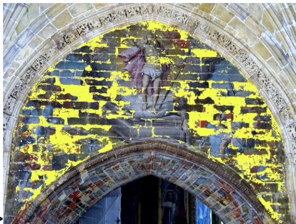
Figure 1. Result of a Maximum Likelihood Classification for the lacunae in a wall painting.
