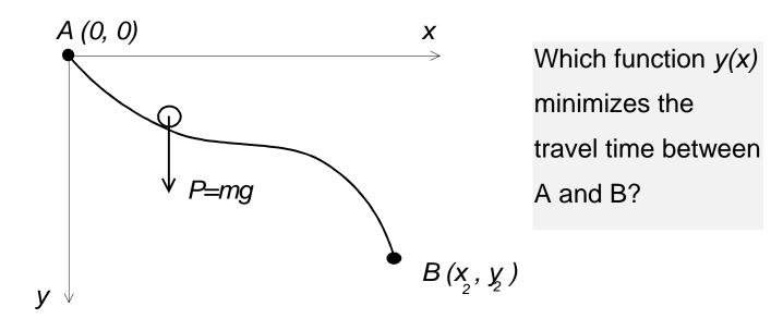
**Computing the travel time assuming**  $y(x) \quad 0 \le x \le x_2$  known Without friction, the increase of kinetic energy is equal to the loss of potential energy, and  $\frac{1}{2}mv^2 = mgy$  or  $v(x) = \sqrt{2gy(x)}$
