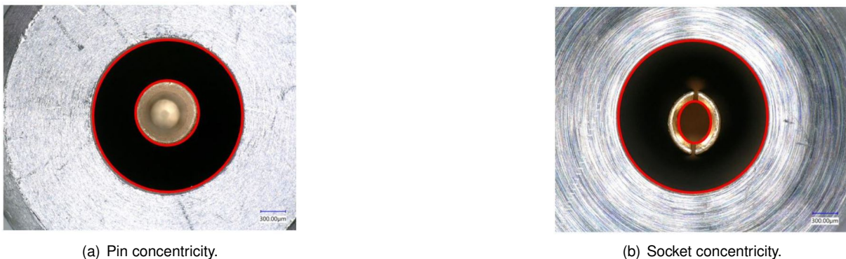
Figure 3.6: Demonstration on how concentricity is calculated.
