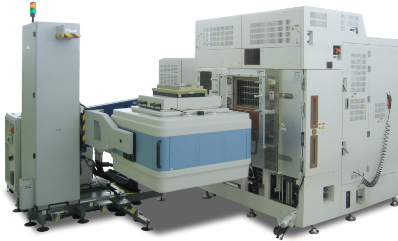
Figure 1.1: Example of an ATE test cell for DDR testing composed of an ATE system and a robotic handler that inserts the packaged integrated circuits into the ATE system (256 units in parallel).
