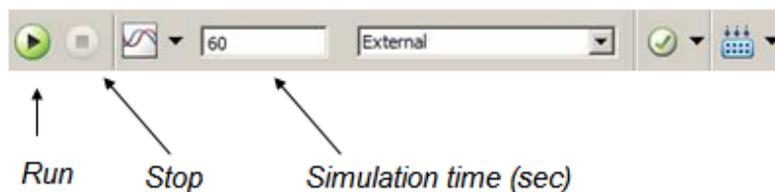
Fig. 7 – Buttons in the SIMULINK project.
