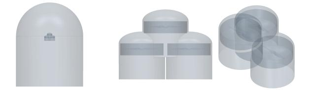
Figure 4.20: Total computational volume (left) along with refinement and rotating volumes (right) in STAR-CCM+ CAD viewer for d = 160 mm and h = 150 mm with APC  $10 \times 6E$  used in both front and back rotor planes
