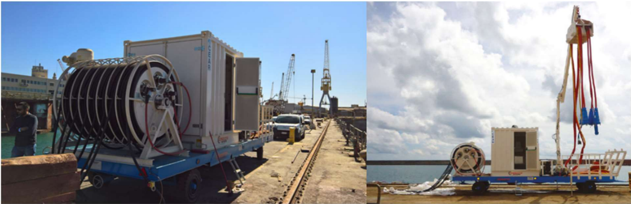
Figure 5 Cable Reel and movable system [15]
