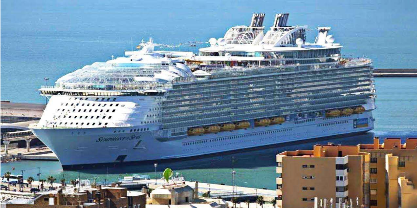
Figure 7 Cruise Ship at berth (Symphony of the Seas length 362 m; gross tonnage 228 000)
