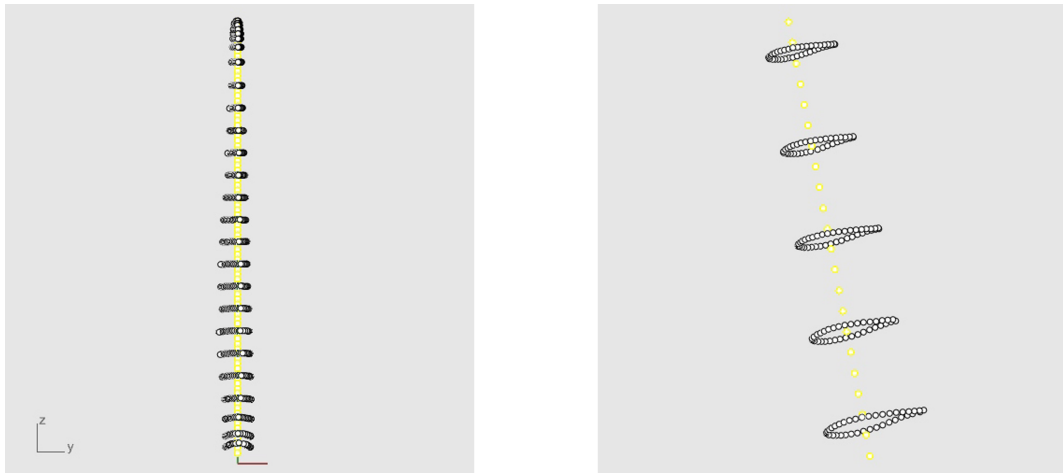
Figure 6.7: Beam grid (in yellow) and outer mesh (white dots) used for the conception of the structural model of the rotor's blade of the DTU 10 MW. Images extracted with Rhinoceros3D®.
