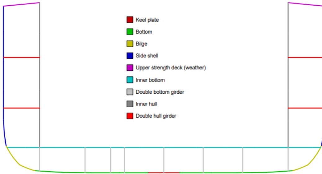
Figure 3.2 - Division of section by panels.
