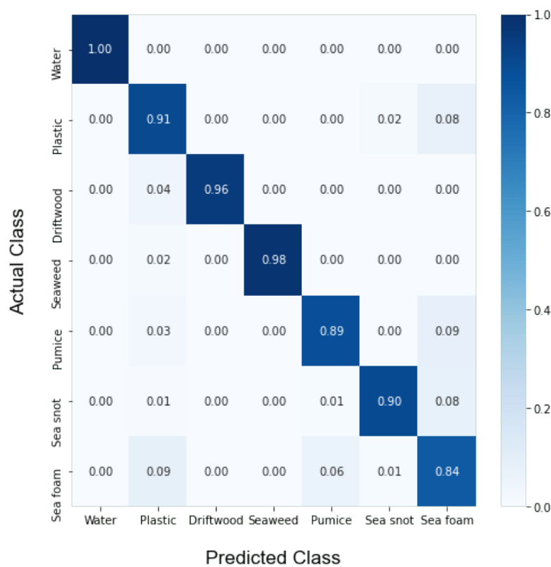
Figure 4.12: Normalised confusion matrix of an XGBoost model trained with 1434 synthetic pixels from each class (10038 pixels in total) generated from a WGAN and that passed the quality filter.
