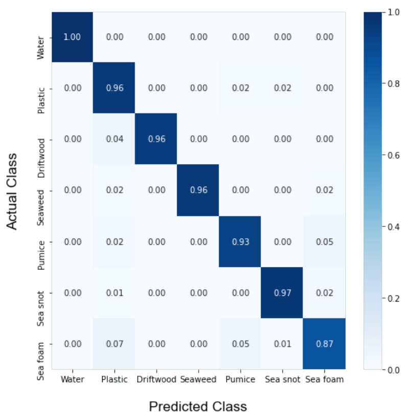
Figure 4.4: Normalised confusion matrix of the XGBoost model trained with spectral bands and all the spectral indices.
