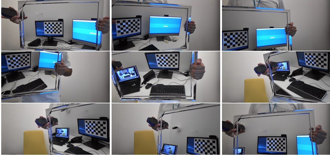
Figure 3.4: Example of the 9 pictures taken to serve as input of one of the extrinsic calibration procedures performed
