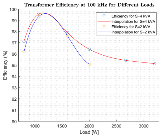
Figure 13: Comparison between transformer efficiency at f = 100 kHz for S = 2 kVA and S = 4 kVA , obtained in the laboratory.
