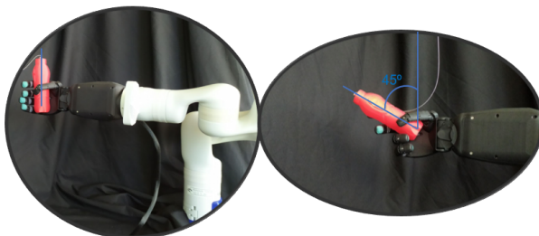
Figure 2: In-hand manipulation task explored in this article - initial state (left) and goal state (right)
