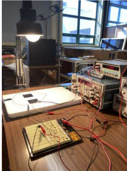
Figure 4.12: Experimental setup to obtain the baseline I-V curves of the Mono-Si cells.
