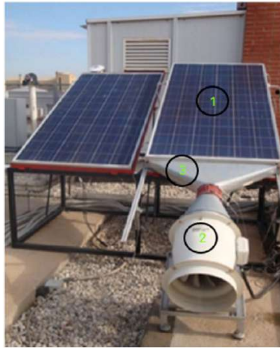
Figure 2.6: PV/T system cooled by forced air circulation [3].
