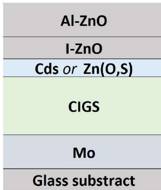
Figure 3.1: CIGS cell model (levels not at scale).
