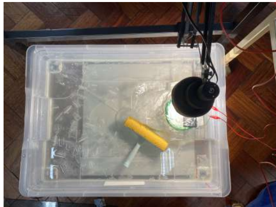
Figure 4.15: Experimental setup to obtain the I-V curves of the Mono-Si cells floating on water and ice.
