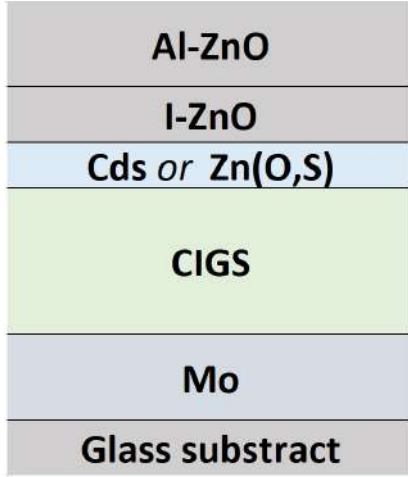
Fig. 2. CIGS cell model (levels not at scale).
