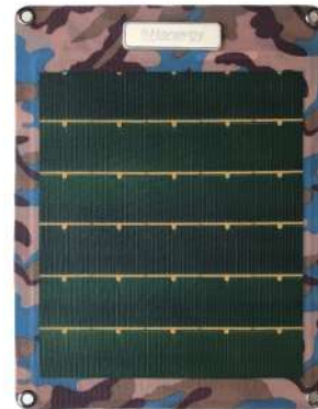
Fig. 3. CIGS panel used to perform the experiments.
