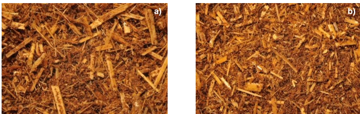
Figure 4.4 a) Nām Substrate grinded with a 10mm sieve; b) Nām Substrate grinded with a 6mm sieve.
