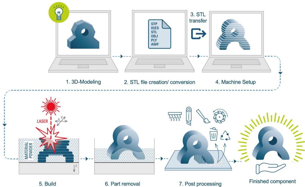
Figure 2.16 – Main steps for a general AM process, adapted from [85]
