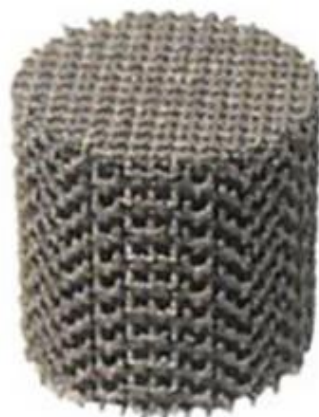
Figure 2.43 – Iron lattice structure [60]
