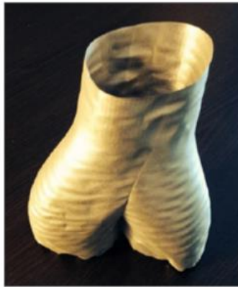
Figure 2.25 – Ni718 manifold showing buckling effect [79]
