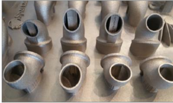
Figure 2.31 – Impact of different part positions and orientations on support structures [79]
