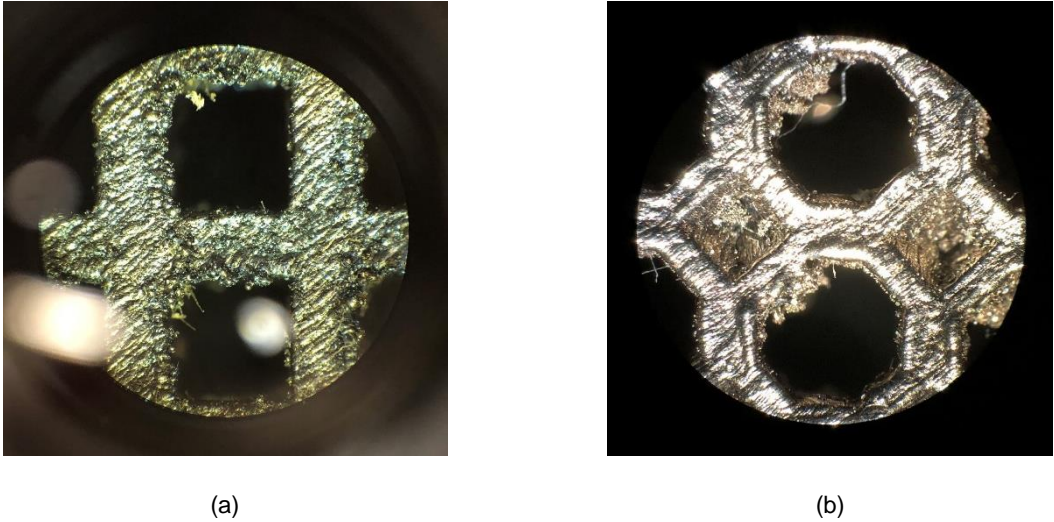
Figure 4.11 – Defects found on the lattice structure of topology: (a) C and (b) TC; (c) shows the average strut size measured for each topology
