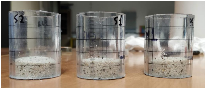
Appendix Figure 5- Equilibrium moisture content test, a) samples; b) hygrometer; c) precision balance Kern ABJ-NM ABS 80-4N.
