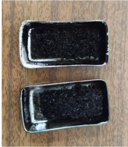
Appendix Figure 4- Crucibles with pine biochar resulting from the horizontal electrical furnace
