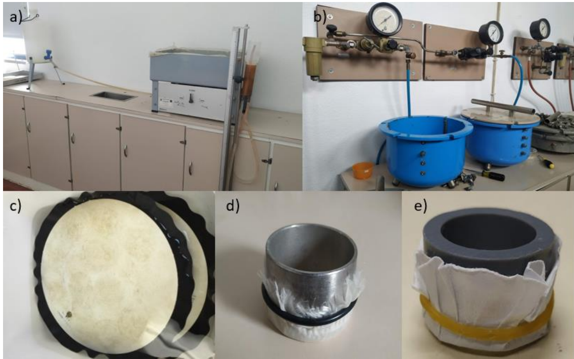
Figure 22- a) Sand suction table; b) Pressure Vessel and air regulator system; c) Ceramic Plates; d) Steel Ring; e) PVC ring
