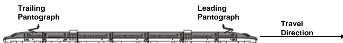
Figure 4.13: Multiple pantograph operation
