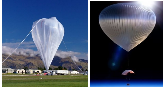
(a) Zero-pressure balloon before launch [6] (b) Zero-pressure balloon at flight [7]
