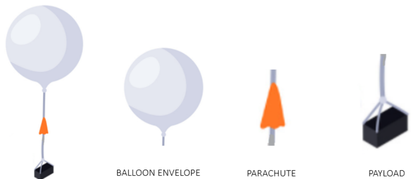
Figure 1.2: Weather balloon usual components.
