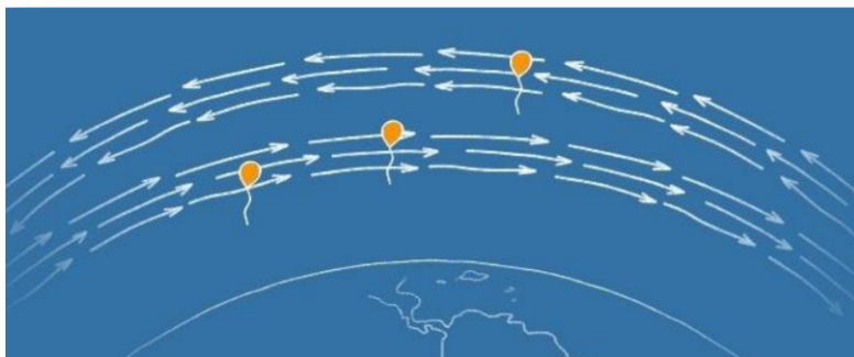
Figure 4.1: Using the wind current directions as lateral movement guidance through altitude control of a weather balloon. Image from the discontinued Google project LOON [35].
