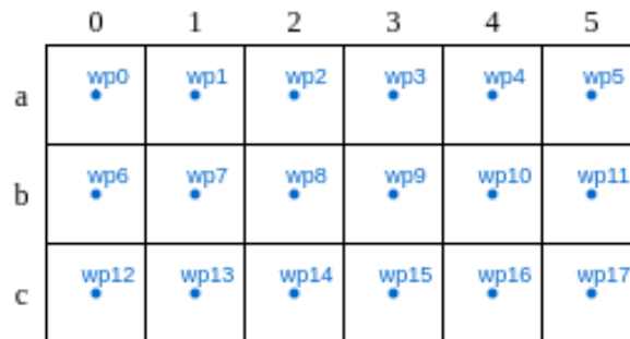
Figure 3.3: The 2D ISS corridor approximation with a waypoint for each location as well as the used nomenclature for each location (the rows are identified by letters and the columns by numbers, so the location containing wp0 , for example, is location a0 )
