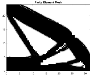
Figure 6: Topology optimized design with AMR for a refinement criterion of 0.2 – 0.8.
