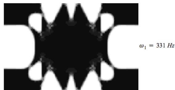
Figure 2.7: Optimized topology for maximization of the fundamental eigenfrequency of a simply supported Mindlin plate with 10% non-structural mass at the center and volume fraction of 60%. Reprinted from Bendsøe and Sigmund [12, p.75].
