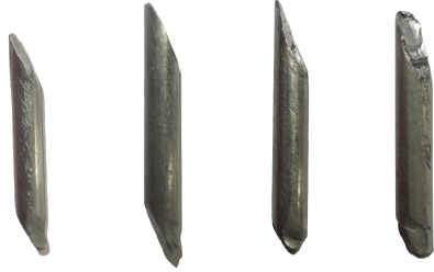
Figure 10: Pure aluminium (Al 99,999%) billets after ECAP: (left to right) 1 pass; 2 passes; 4 passes; 8 passes
