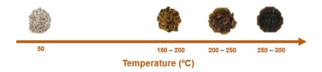
Figure 1.2: Biomass torrefaction severity in regard to the temperature; raw biomass, mildly torrified biomass, medium torrified biomass and severe torrified biomass.
