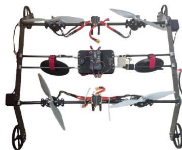
Figure 6.19: BogieCopter with two 1 kg weights, simulating a 2 kg payload.
