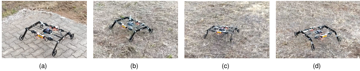
Figure 6.10: BogieCopter moving on rocky soil ground: (a) Test starting in a sidewalk (b) Longitudinal motion (c) Turning (d) Climb of small slope ( \sim 5^\circ ).
