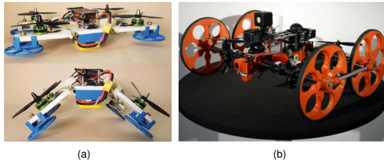
Figure 2.12: Four-wheeled passive actuated MAVs: (a) Flying STAR [56] (b) Inkonova Tilt Scout [57].
