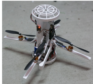
Figure 2.6: Morphing two-wheeled quadrotor [40].
