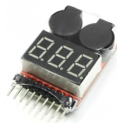
Figure E.2: Battery cell tester and alarm.
