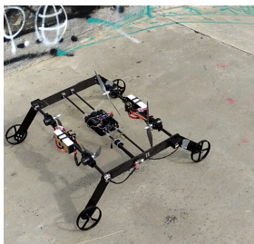
Figure 6.12: Climb of a 14^\circ slope in normal mode.
