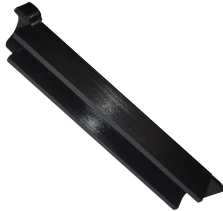
Figure 4.13: Simple assembly jig fabricated to assemble the battery supports at the right orientation and distance from the motors support.
