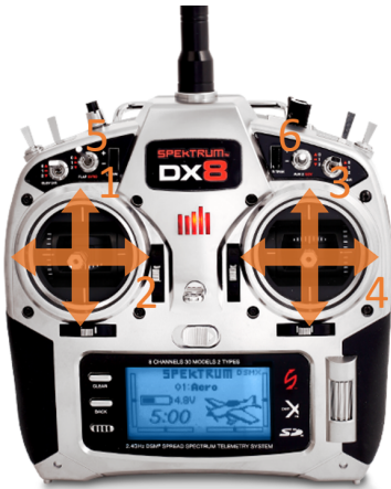
Figure 5.8: Spektrum DX8 Mode 2 radio transmitter [156], each stick motion follows the standard: (1) Throttle (2) Yaw (3) Pitch (4) Roll (5) Flaps Gyro (6) Aux 2 GOV.
