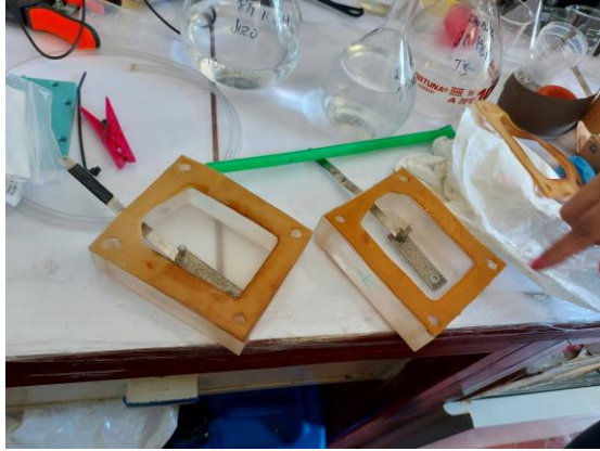
Figure 5 - Solutions compartment, with rubber sealing to avoid liquid leakage. The chosen membrane will be put in the middle. Electrodes are visible inside the compartments.
