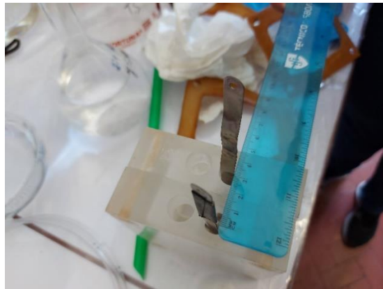
Figure 7 - Average distance between electrodes: 3 cm. Minimum distance 2.5 cm, maximum distance 4.0 cm.
