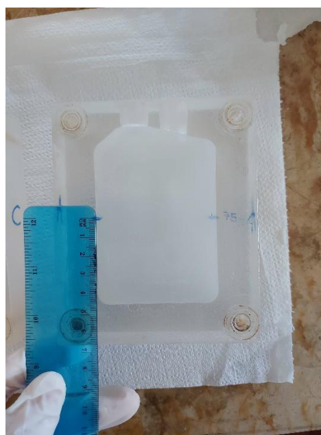
Figure 20 - Active membrane height = 4,5 cm.
