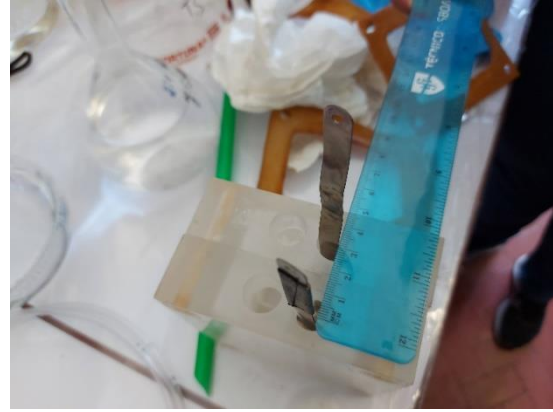
Figure 6 – Average distance between electrodes: 3 cm. Minimum distance 2.5 cm, maximum distance 4.0 cm.
