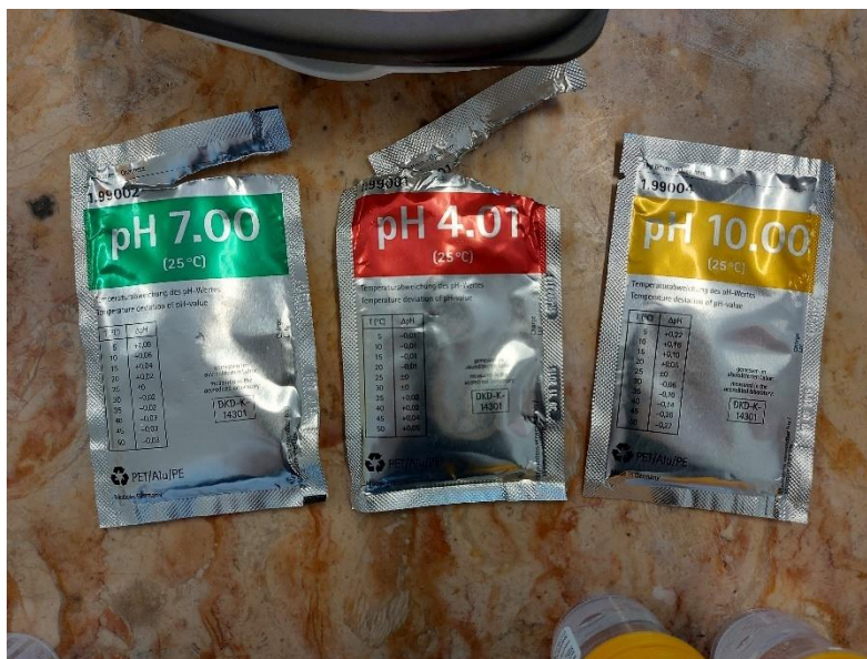
Figure 18 – Standards used for pH calibration.
