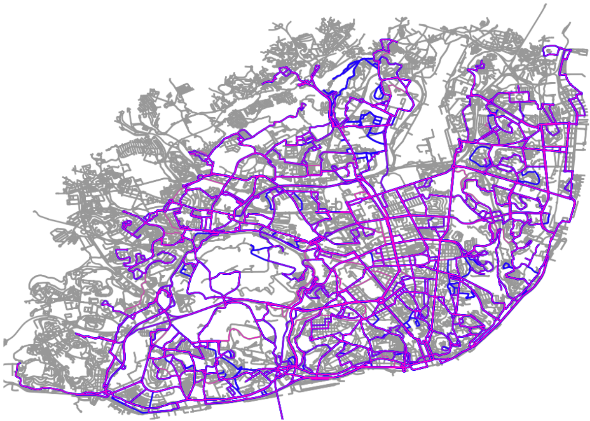
Figure 7.9: Roads covered by the original bus network (in blue) and the best network obtained through optimization (in pink).
