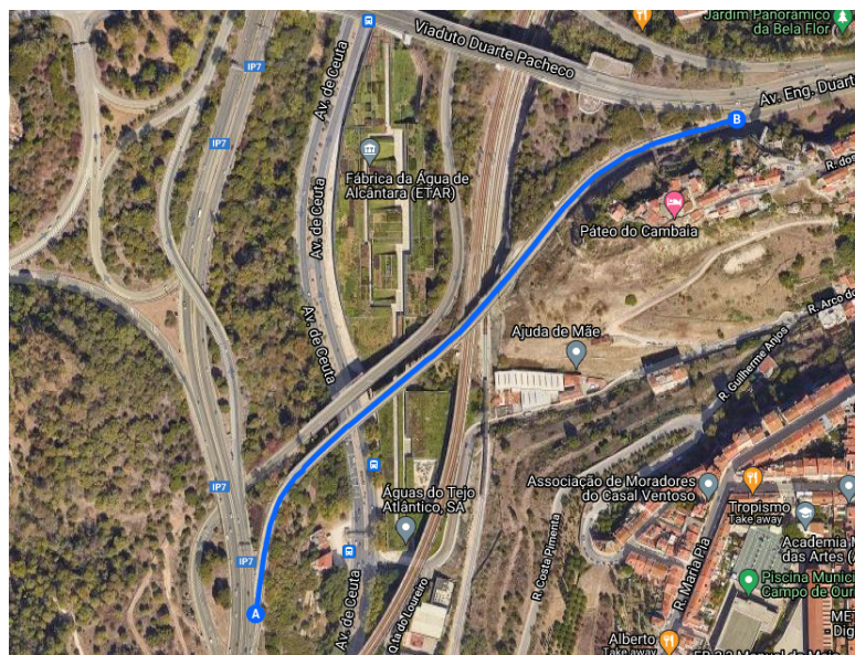
Figure 4.10: A2 exit missing from the network obtained with OSMnx.
