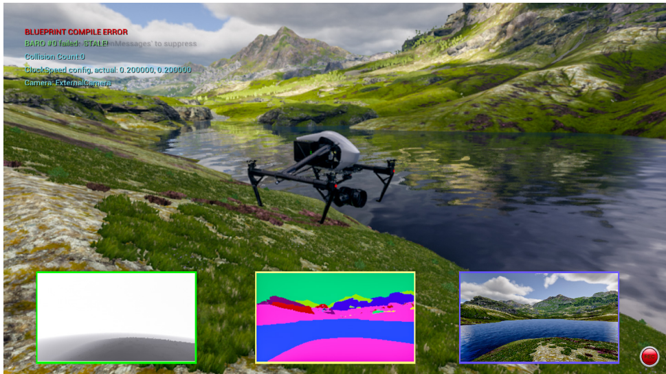
Figure 3.5: Snapshot that shows two aerial vehicles flying in a rural environment. The inset shows depth, object segmentation and front camera streams generated in real-time.
