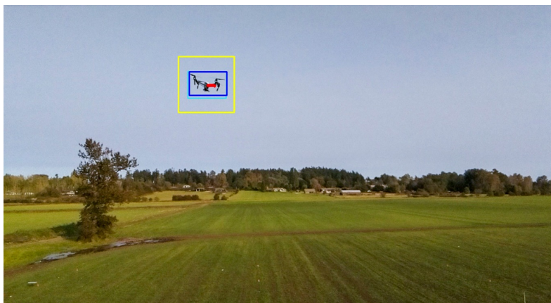
Figure 3.2: Example of an output of the previously proposed system. LiDAR detections are identified by red dots, the ROI, ground truth and YOLOv3 detections correspond to the yellow, light blue and dark blue bounding boxes, respectively. Taken directly from [18].
