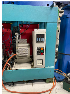
Figure 14: Electric Oven and controller
