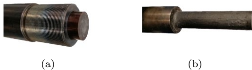
Figure 9: Bar ends with compression rods: (a) Short Rods; (b) Long Rods
