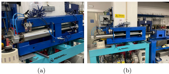
Figure 12: Moving Actuator Selector: (a) High and medium speed configuration; (b) Quasi-Static configuration
