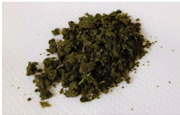
Figure 3.1: Sample of Ulva lactuca residues after protein extraction as described in subsection 3.2.1 . The particle's size varies from approximately 1 mm to 60 mm. Throughout this work, residues with no more than 11 mm were used, as depicted above.
