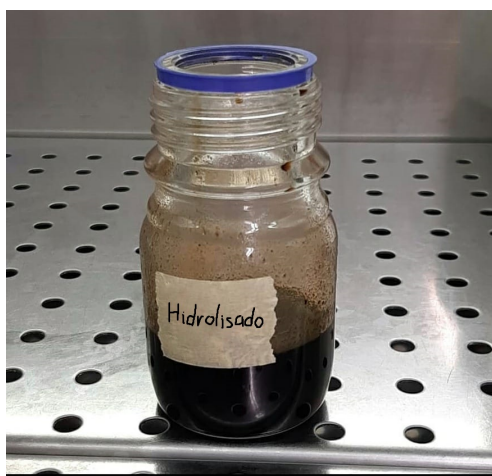
Figure B.2: Concentrated hydrolysate used in the P3HB production assays
