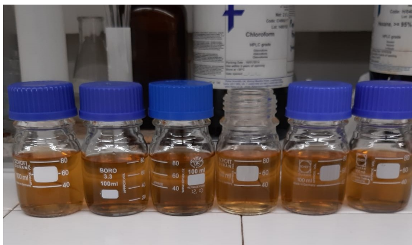
Figure B.1: Centrifuged and filtered hydrolysate after scaled-up combined hydrolysis distributed among the 6 Schott flasks right before the concentration step
