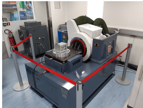
Figure 3.16: Shaker at ESA ESEC facilities.
