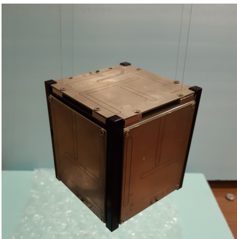
Figure 5.3: Test set-up: fishing line SP testing configuration.
