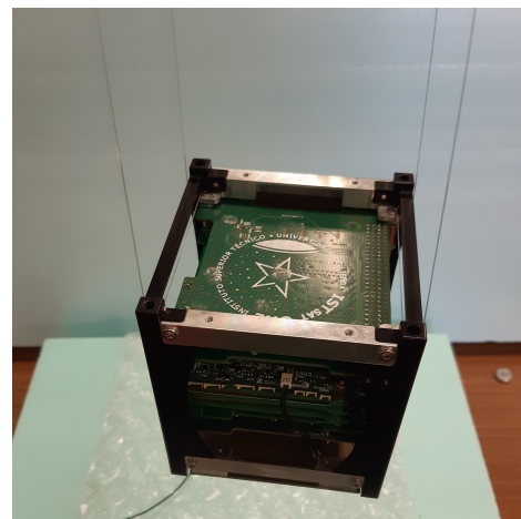
Figure 5.4: Test set-up: fishing line PL testing configuration.
