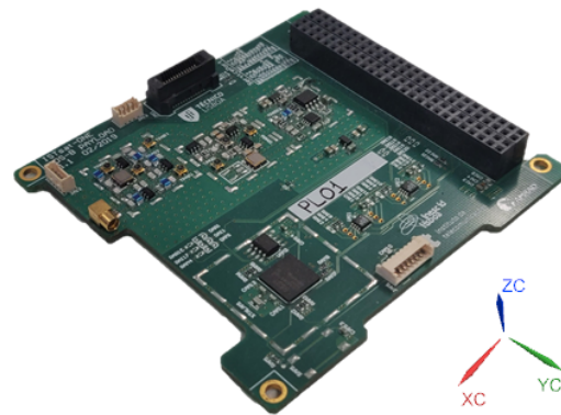
Figure 4.7: ISTSat-1 PL board.
