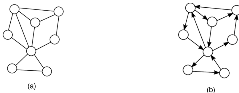
Figure 2.1: (a) An example of an undirected graph and (b) an example of directed graph. Adapted from Fionda and Palopoli (2011).
