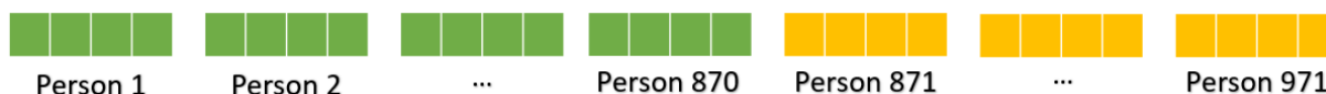
Figure 5.3: Division of the CUHK01 dataset between training and testing. Each square represents an image and in this case each person has 4 images so each one has 4 squares. The green colour represents the training set that are all people from 1 to 870. The yellow colour represents the test set, from 871 to 971.
