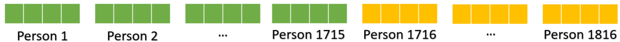
Figure 5.4: Division of the CUHK02 dataset between training and testing. Each square represents an image, in this case each person has 4 images so each one has 4 squares. The green colour represents the training set that are all from 1 to 1715. The yellow colour represent the test set, from 1716 to 1816.
