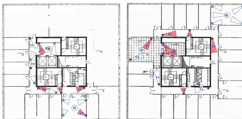
Figure 1.1: A Closed-circuit Television map in two floors of Torre Norte - Instituto Superior Técnico.
