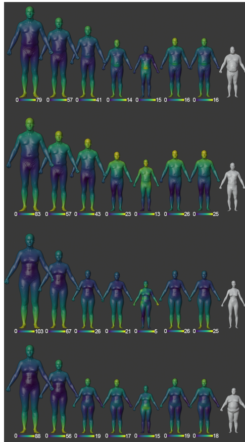
Figure 5.4: Error color map of the pca model using several body measurements sets. Each column corresponds to a subset of the top 10 body measurements represented in Table 4.6 or from the selected 7 from Table 4.7, from left to right: (a) top 2 (b) top 4 (c) top 6 (d) top 8 (e) top 10 (f) selected 6 (g) selected 7 (h) original shape. The yellow parts correspond to the parts that have a higher distance error in cm associated, while the dark blue parts are the ones that are more similar to the original shape.
