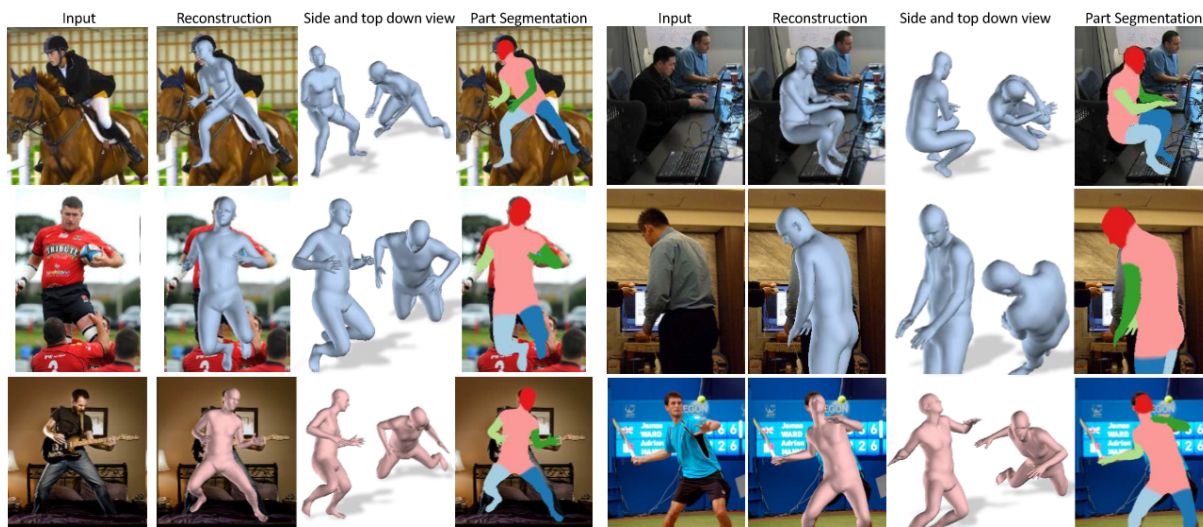
Figure 3.4: Human Mesh Recovery (HMR): End-to-end adversarial learning of human pose and shape. The authors describe a real time framework for recovering the 3D joint angles and shape of the body from a single RGB image. The first two rows show results from our model trained with some 2D-to-3D supervision, the bottom row shows results from a model that is trained in a fully weakly-supervised manner without using any paired 2D-to-3D supervision. They also infer the full 3D body even in case of occlusions and truncations.
