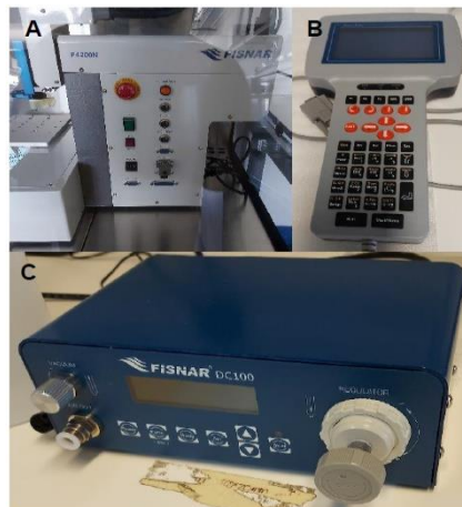
Figure 14 - Bioprinter setup; A: Fisnar Compact Desktop Robot; B: Teach Pendant; C: Air dispensing Unit
