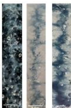
Figure 28 - Pictures of singles strands of sisECM (left), sisECM + 0.05% PEDOT:PSS (center) and sisECM + 0.1% PEDOT:PSS (right); scale bar 5 mm.
