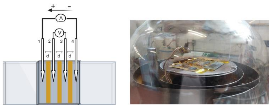
Figure 12 - 4-probes schematic (left), with the representation of the 4 probes (current passes on the outer probes and voltage is read across the inner probes) and gold deposited strips, with d corresponding to the gap between gold strips; and gold deposition chamber (right)
