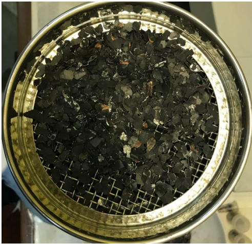
Figure 49 - Sieved non-treated material after first crushing for sieve 2.8 mm.
