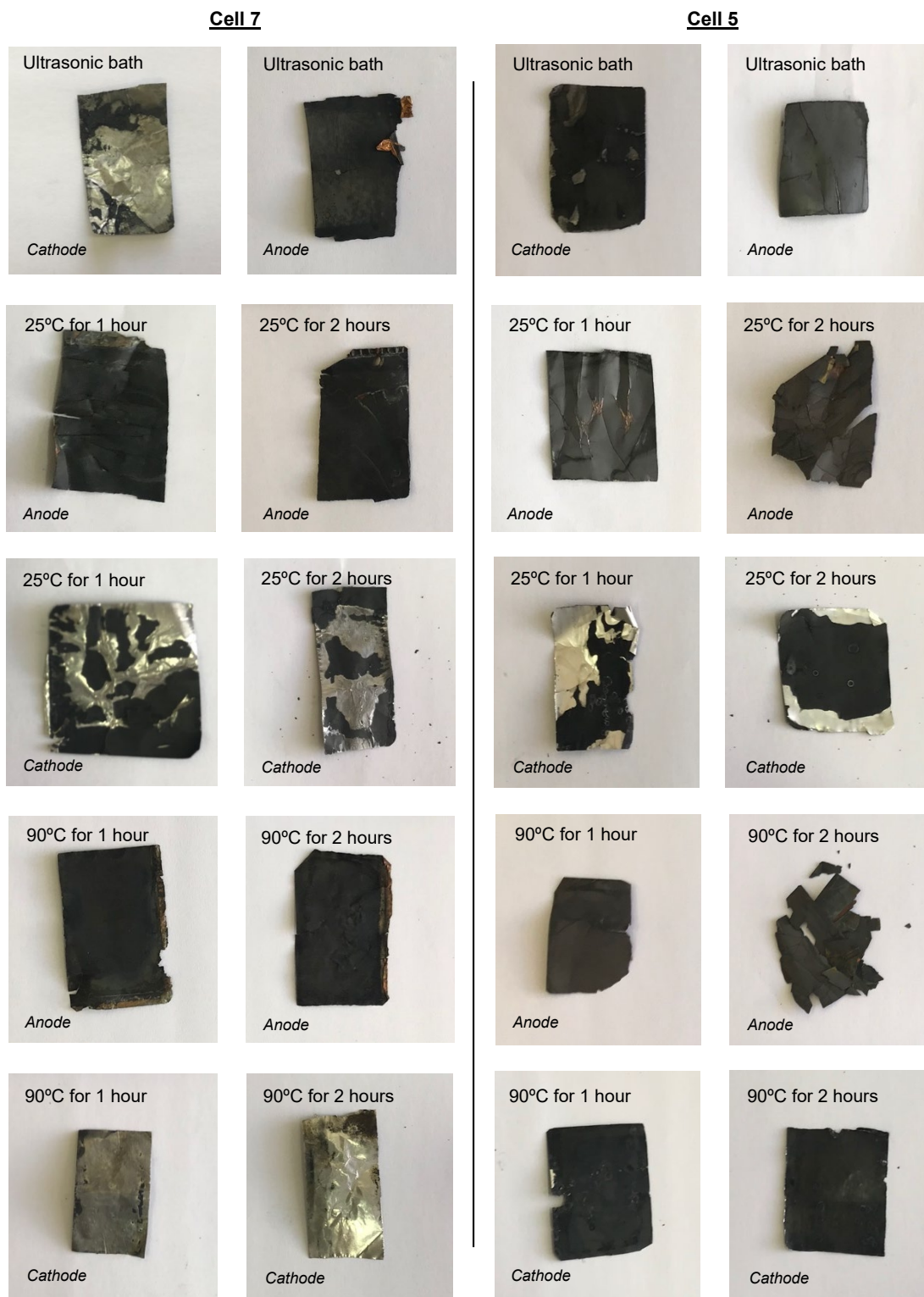
Figure 40 - Electrode samples after solvent dissolution and manual brushing.
