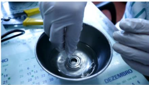
Figure 9. Grease removal process from the bearings.
