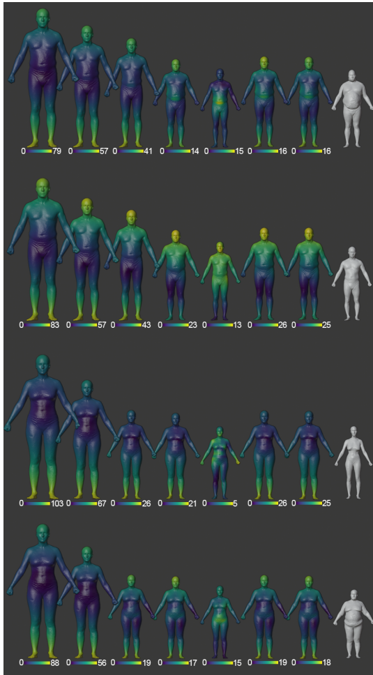
Fig. 1. Error color map of the pca model using several body measurements sets. Each column corresponds to a subset of the top ten body measurements or from the selected seven from Table 4, from left to right: (a) top two (b) top four (c) top six (d) top eight (e) top ten (f) selected six (g) selected seven (h) original shape. The yellow parts correspond to the parts that have a higher distance error in cm associated, while the dark blue parts are the ones that are more similar to the original shape.
