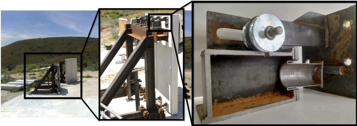
Figure 3.4: Representation of a section cut from the Energy Absorption Device (EAD), within the protection system [27].
