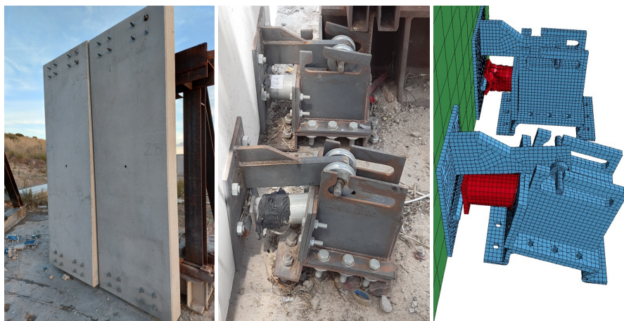
Figure 4.26: Representation of the experimental setup versus the first generation of models (May, 2021) created with Semi_Restricted_System [27].
