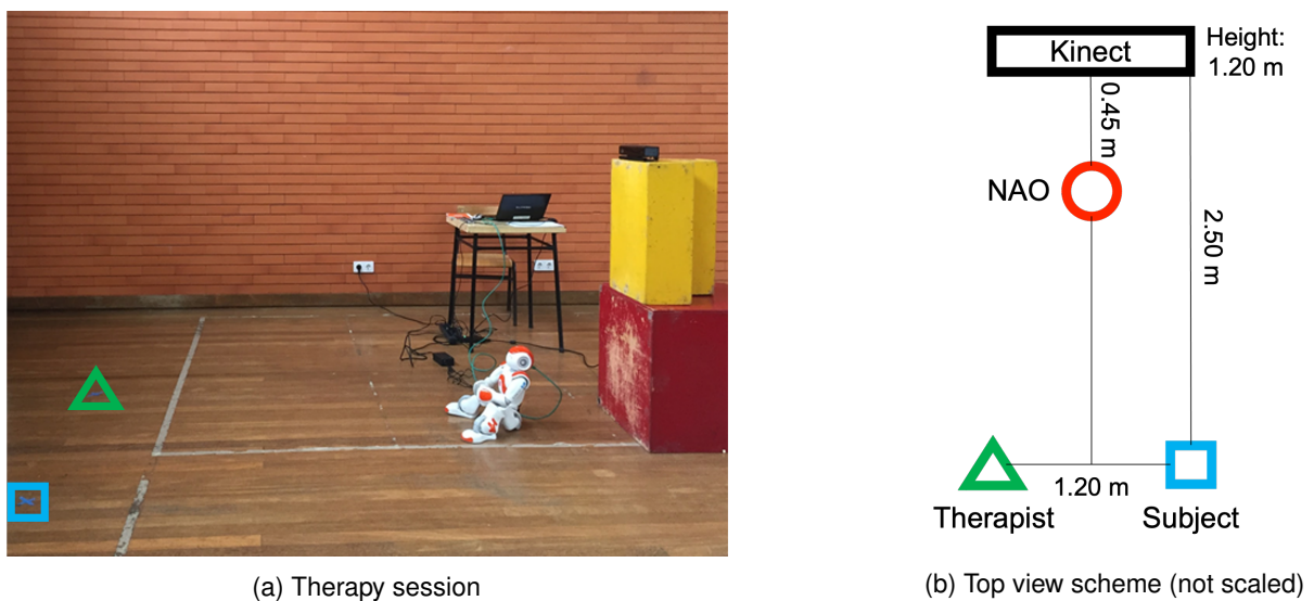
Figure 3.2: Pilot study setup. The therapist is represented by a green triangle, the ASD subject is represented by a blue square and NAO is represented by a red circumference
