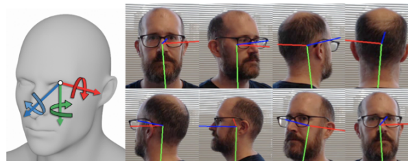
Figure 2.9: Head pose estimated coordinates, parameterized by pitch (red-axis), yaw (green-axis) and roll (blue-axis) (extracted from [8])
