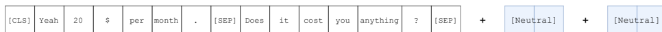
Figure 4.3: Example of the input of the classification layer of the reply sentiment prediction model with information from the labels of the context sentences. This method involves concatenating vector representations of the sentiments corresponding to the context sentences.
