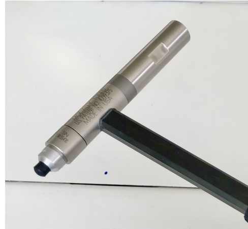
(b) Impact hammer with soft tip and extra mass added.
