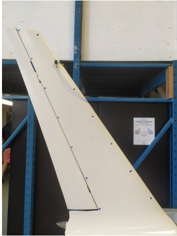
(a) Marks and sensors on winglet.
