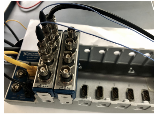
(b) DAS setup for tests on morphing wing.
