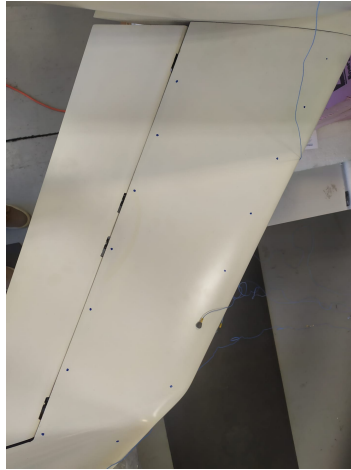
(b) Marks and sensors on horizontal stabilizer.
