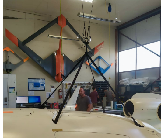
(b) Connection between aircraft and cables.
