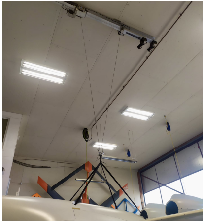
(a) Mechanism to hang aircraft from ceiling.
