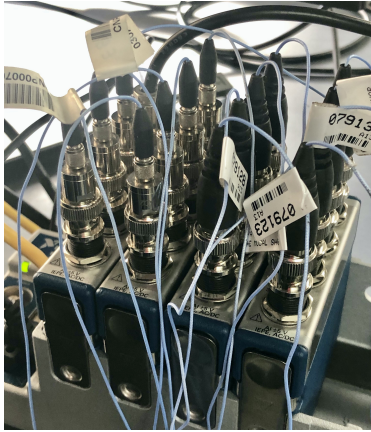
(a) DAS collecting data from 15 sensors and impact hammer.
