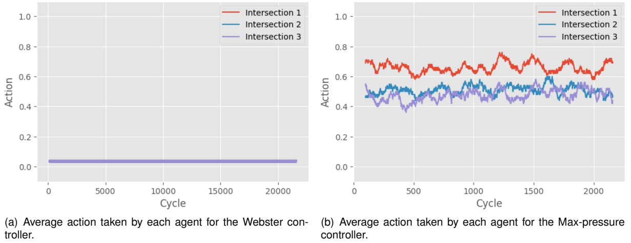
Figure 6.1: Average action taken for the Webster and Max-pressure controllers in the arterial network, where action 1 represents changing to next phase and action 2 represents keeping the current phase active.
