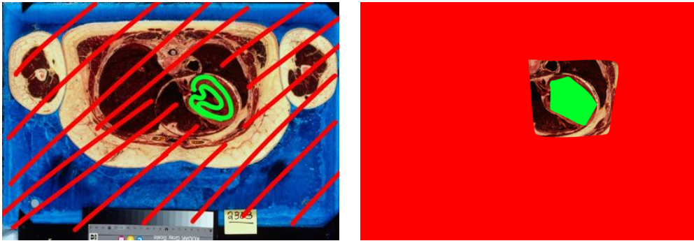
Figure 4.2: Examples of the first inputs explored for the algorithm 2 represented in (a) and (b). The object being contoured is the left ventricle of the heart of slice number 2292. The colors red and green represent sure background and sure foreground respectively.
