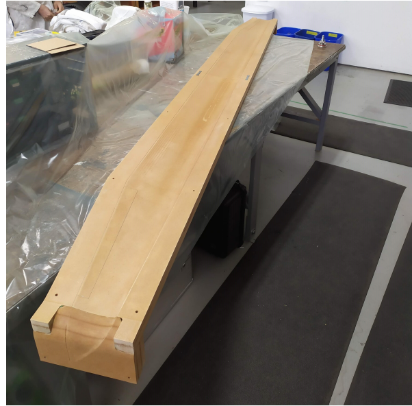
(b) Upper surface molds.
