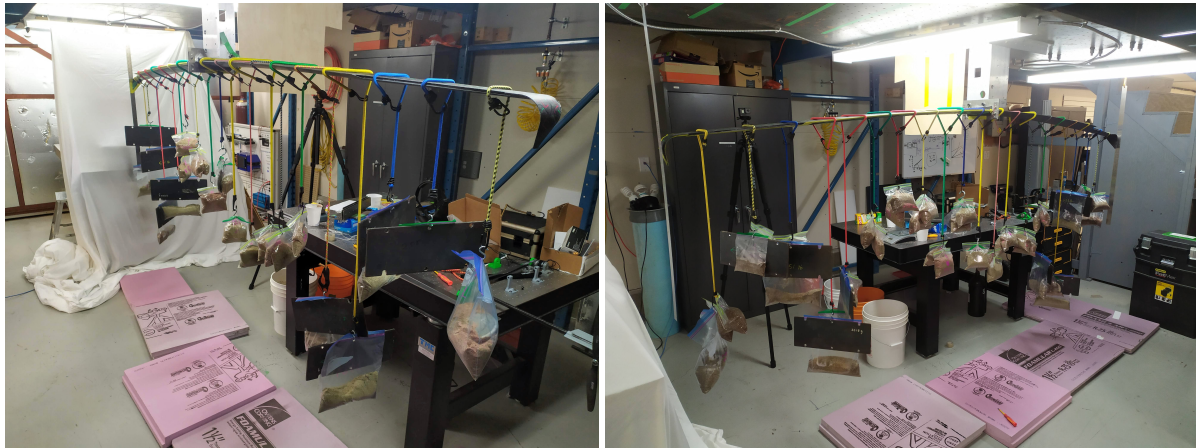
(a) Photograph of 3g loading condition.
