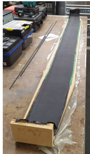
(b) Lower surface after cure resting on the mold.
