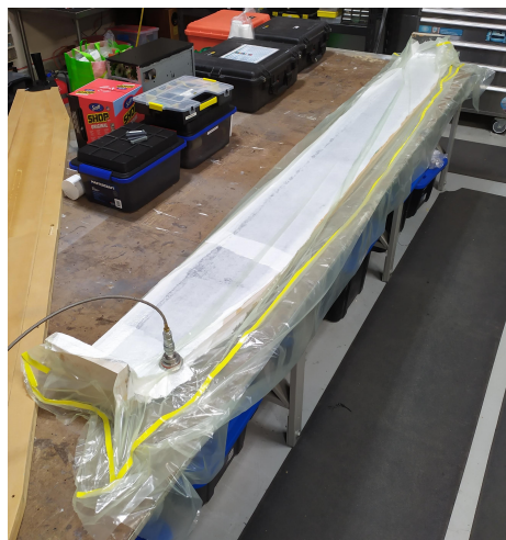
(a) Lower surface curing under vacuum.
