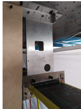
(b) Wing support to the ceiling.
