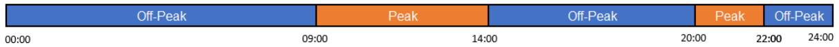
Figure 7 – Saturday periods defined by ERSE for weekly cycle tariffs during summer time
