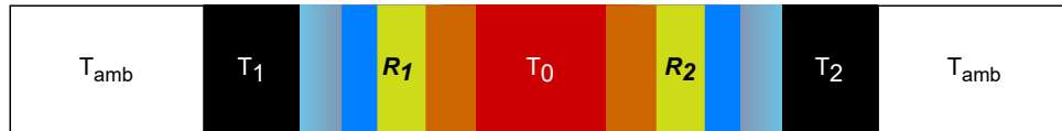
Figure 3.4: Thermal system of the flow channel where the sensor will be placed when there is no flow.
