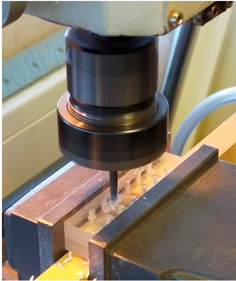
(a) Milling of the fluid channel.
