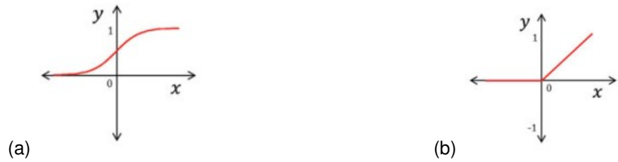
Figure 2.5: Activation functions, (a) illustrates the Sigmoid function and (b) illustrates the ReLu. [19]
