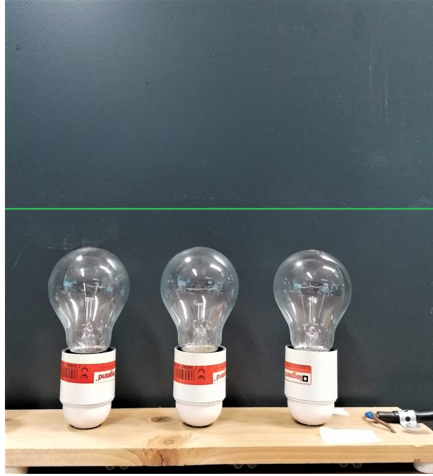
Figure 4.5: Simulation of the atmospheric turbulence: three 100 W lamps heat the uplink beacon propagation region, causing disturbance of the beam.
