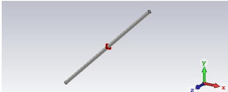
Figure 3.8. Design of the slanted half-wavelength dipole antenna in CST, placed in the  $xOy$  plane.
